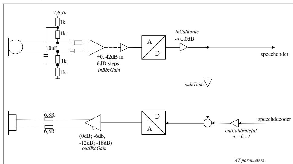
Figure 1: AT audio programming model
